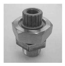
The Insertion Adapter mounts Model 399VP into a 1-1/2 inch NPT process pipe. Unscrewing the hex nut allows easy sensor removal without twisting the sensor cable.
